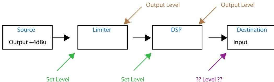
Two processing stages are added between the source and destination. Note the points where input and output levels need to be set.
