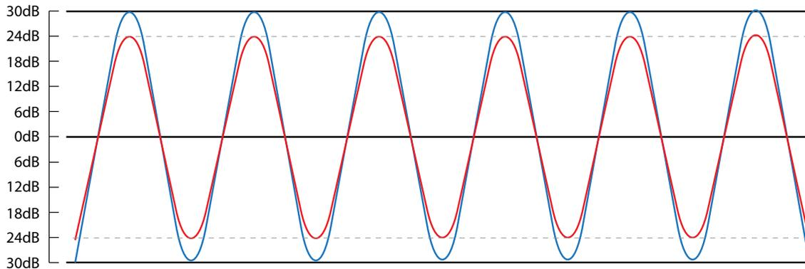
**The blue line indicates a maximum +30dBu input signal level sent into the audio device described above. The device's resulting +24dBu output, shown in red, is 6dB softer.**
