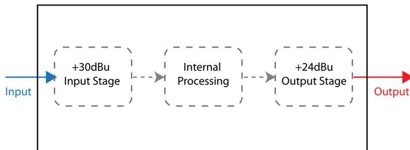
An audio device designed with a 30dBu maximum input stage and a +24dBu maximum output stage
