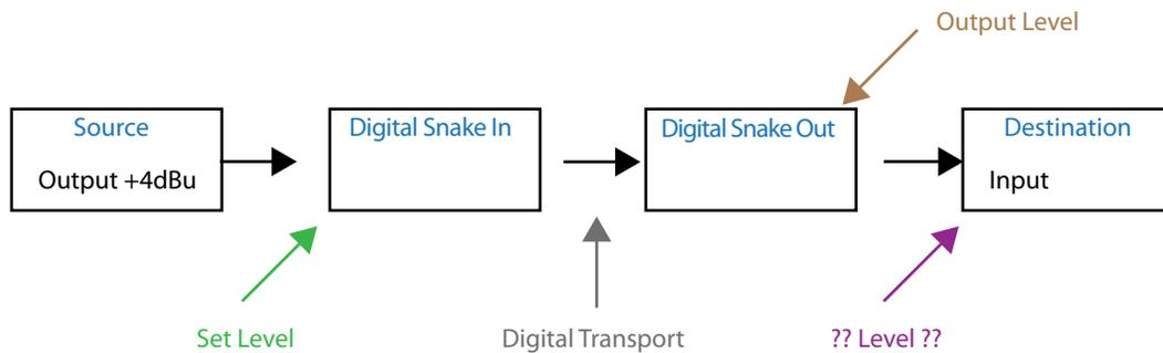
A digital snake replaces the processing devices; note where the I/O levels need to be set.
