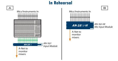
*Figure 2.* There are two basic ways to get your audio into the system. If you already have a console you like, you can connect its outputs to the AN-16/i Input Module (A). Or, using the AN-16/i-M Mic Input Module, you can connect your mics and instruments directly (B).
