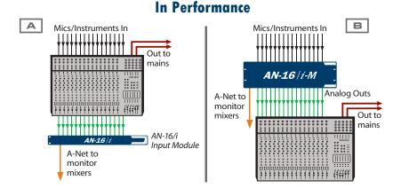
*Figure 3.* Moving to the gig is easy. Either connect the console you're already using to your main effects and amps (A), or connect the analog outputs (mic split or direct out) on the AN-16/i-M to your console (B).
