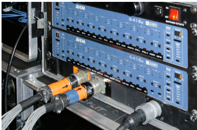
6416o Output Modules on tour with Luke Bryan
