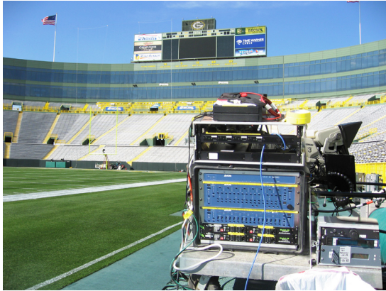
Aviom 6416m, 6416o v.2, and MH10f in a remote rack
