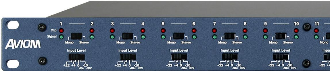
The AN-16/i v.2 input channels can be thought of in stereo channel pairs. The A360 default routing uses odd numbered input channels for left or mono and even numbered input channels for the right side of a stereo channel.
