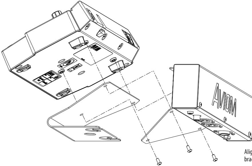
Align the screw holes in the MT-X and MT-1 and secure both brackets to the Personal Mixer using the screws provided.
