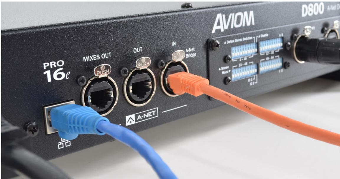
The Wi-Fi router is connected to the Ethernet port on the D800 rear-panel.
